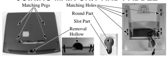
Match the matching pegs on the back of the main unit against one of the two sets of matching holes on the paddle. It is recommended to hook on the lower set of holes for better stability. First aim the matching pegs toward the upper round part of
